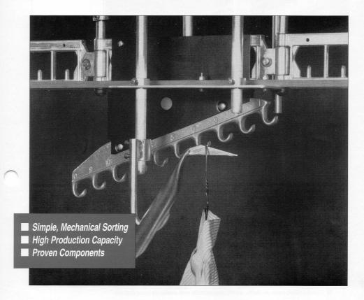
**Dispat-U-Veyor** is the leader in basic mechanical sorting conveyor systems. With a capacity of handling 1,200 loads per hour, sorting up to 60 stations, the DT has a 25-year record of success. A **DISPAT-U-VEYOR** system is easily applied in any garment handling operation, and can be used in many light item delivery systems.
